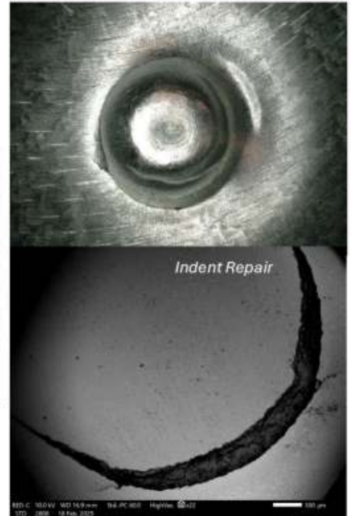
Tangential crack (ring-like)
