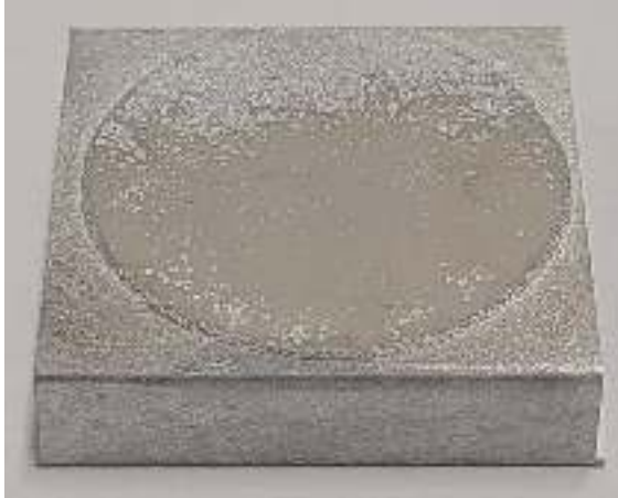
ASTM C633 minimum thickness (0.38 mm)
