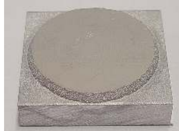
Maximum depth of blend-out repair (1.8 mm)
