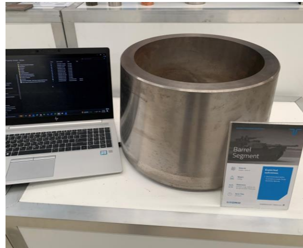
4340 Steel Barrel Segment (circa 34hr spray, 130kg),
