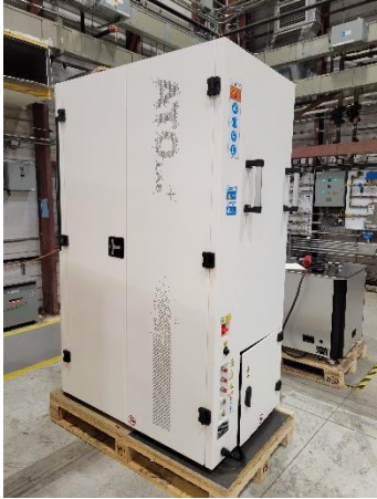
Ultrasonic Atomizer To produce custom powders from rods or wires
