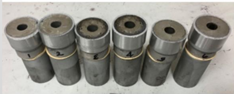
Post-Test, Glue-Less Bond Coupon: Valimet 6061 on EZ33A
